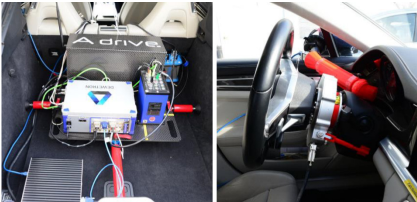
Figure 5a: Measurement Setup: IMU; 5b: measurement steering wheel and AVAD.
